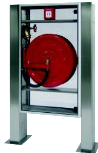
Free-standing cabinet „Special design“ Type 1-C/K-M-LEF-30-2AF-MAK-BS-SO 740 x 1.240 x 280 mm (w x h x d) (Dimensions without rectangular column frame) Cabinet made of stainless steel material-No. 1.4301, visible surfaces polished grain 240. Front and backwall with folding aluminium frame with full macrolon glass panel.
