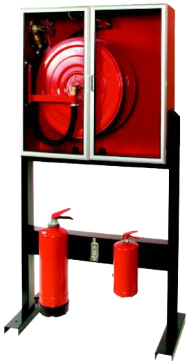
Free-standing cabinet „Special design“ Type 1-C/35-AF-ACR-SO 900 x 900 x 300 mm (w x h x d) (Dimensions without mounting-frame) Front doors with two folding aluminium frames with 3 mm thick acrylic glass panels. Provided with toggle lock. Frame with holders for 3 portable fire extinguishers.
