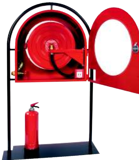
Free-standing cabinet „Special design“ Type 1-C/30-HALBR-FS-AUDI-SO 900 x 900 x 250 mm (w x h x d) (Dimensions without pipe-frame) half-round design made of 3 mm steel sheet, mounted in pipe-frame, colour black. Door and backwall have round windows with acrylic glass panels, 4mm.
