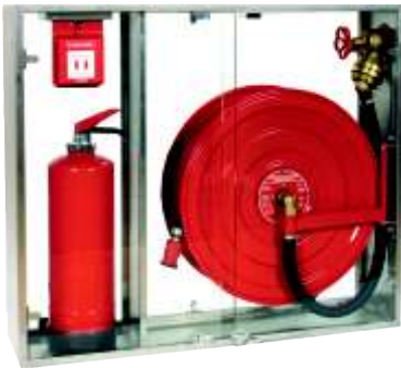
Combi-surface cabinet „Special design“ Type 1-C/K-K-M-30-E-BS-ESG-SO 1.090 x 920 x 250 mm (w x h x d) made of stainless steel, material-No. 1.4301, visible surfaces polished grain 240. Doors and backwall of cabinet consist entirely of ESG glass panel, 6 mm.
